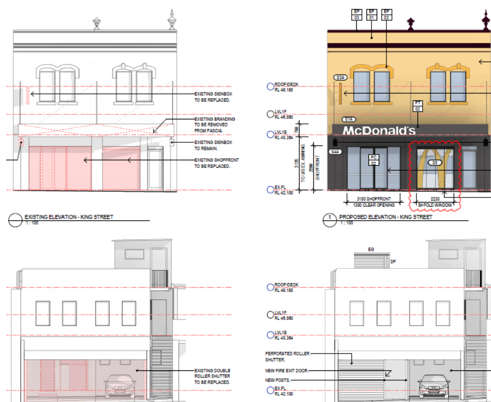
Figure 6: Existing and proposed front and rear elevations
