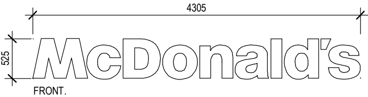
S1A AWNING SIGN NON-ILLUMINATED LETTERING (FLAT / PAINT).
